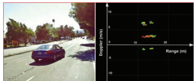
▲ Fig. 4 Range-Doppler profile of a moving sedan, showing a clear difference in the speed of the wheels vs. the vehicle body.
